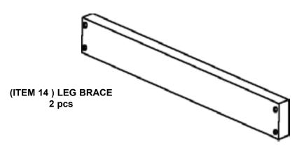
•Attach Leg Braces onto each Side Table assembly using 1/4" x 1" Bolts. Do not tighten bolts completely.
